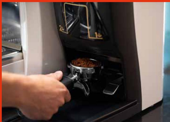
With G10 evo you can also benefit from two grinding solutions. The patented **Dose On Demand** option, which is ideal for locations with high consumption peaks, automatically pre-grinds the next coffee dose. Instead, thanks to the **Grind On Demand** mode, the dose is instantly ground and dispensed just before being served.
